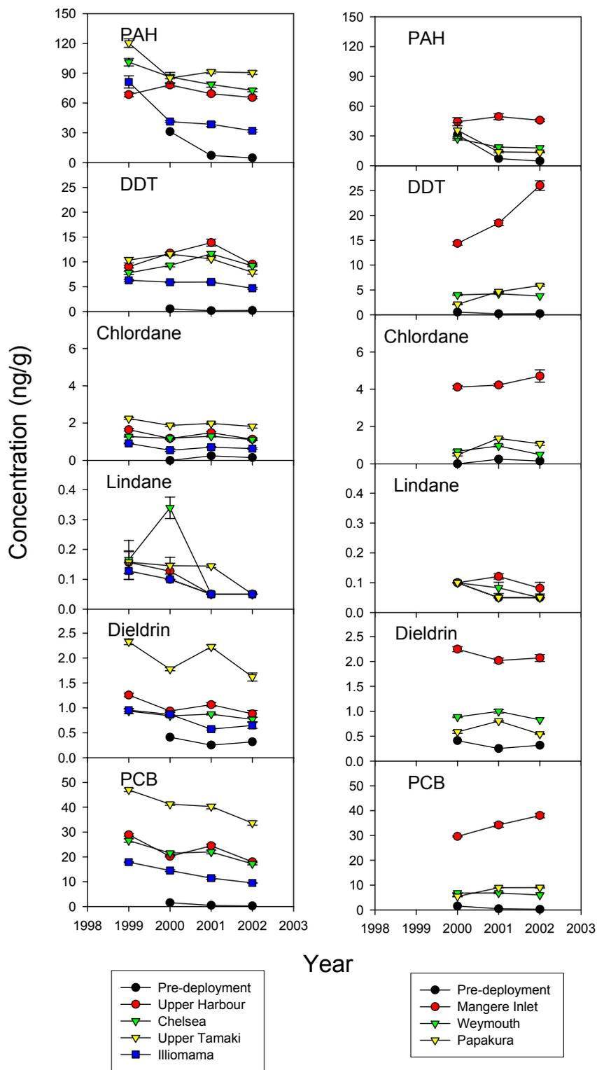
Figure 19: Lipid normalised organic contaminant concentrations (ng / g (lipid)) of mussels trans-located into the Waitemata Harbour (left column) and the Manukau Harbour (right), from 1999 to 2002. Values are also given for contaminant levels in samples prior to deployment. The lower Tamaki site was only sampled in 1999. Data below detection limits (D.L.) and presented as 0.5 x D.L.
